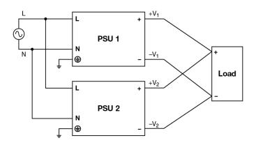
Fig. 10 Parallel Operation Connection Diagram
