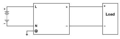
Fig. 12 DC Input Operation Connection Diagram
